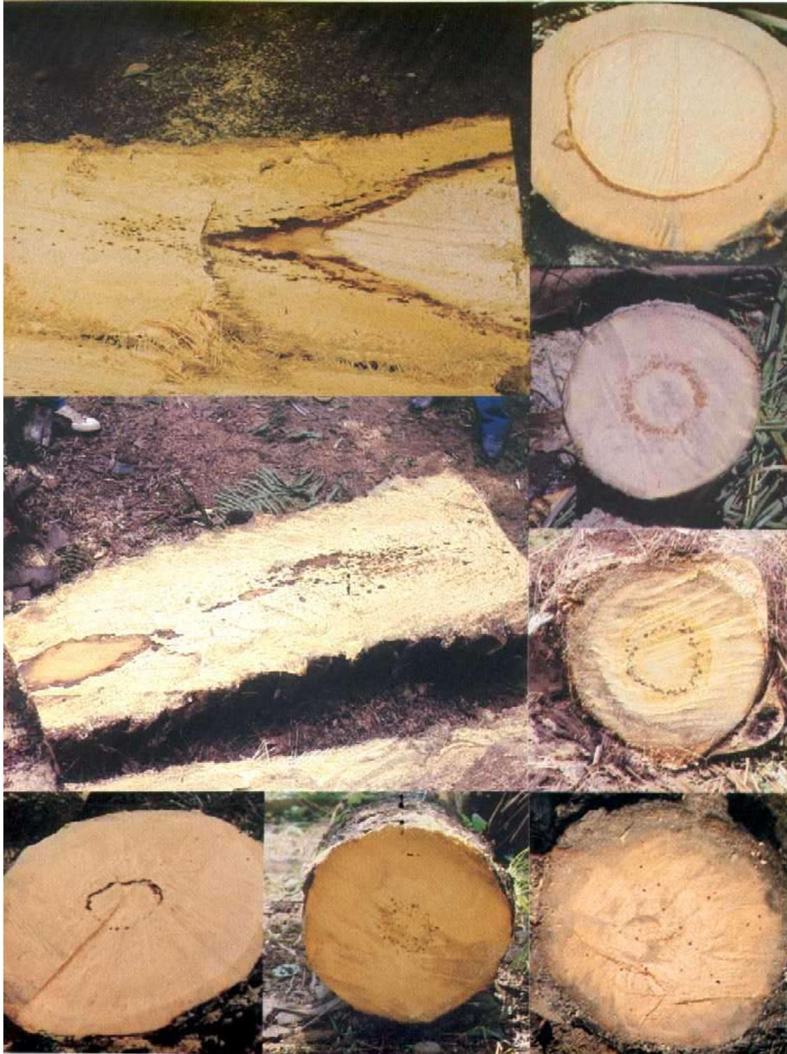
**Fig. 2.** Internal symptoms in oil palm trunks affected by the red ring disease
